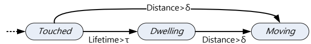
Figure 1. Three phases of a touch point. We set \tau = 450 ms and \delta = 5 mm for our implementation.
